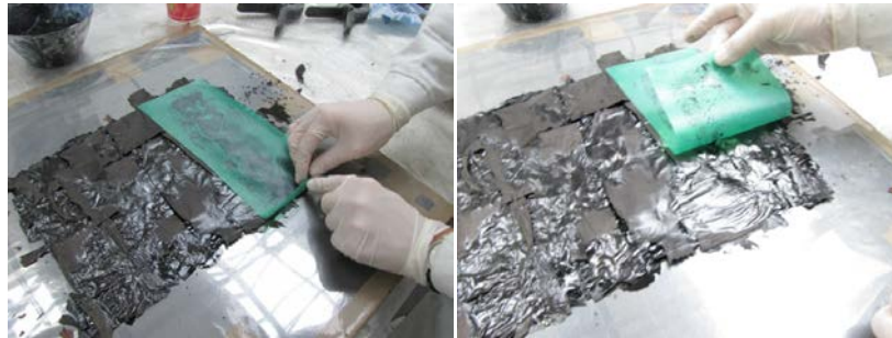
Figure 2.1 Composite preparation from the developed nanofibrous prepreg
