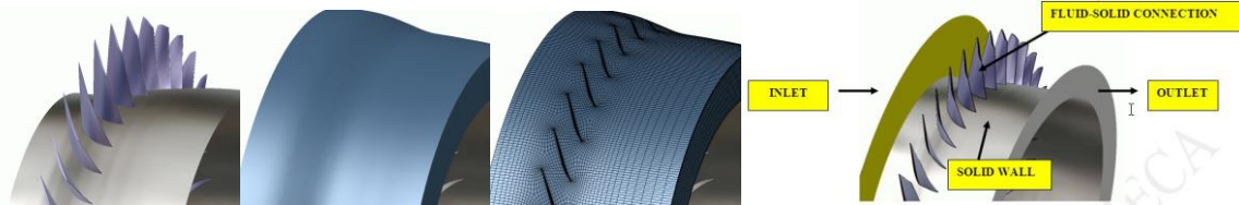
Figure 17: (from left to right) Solid body of the blade; volume between the blades; mesh of the fluid domain; physical properties and multi-physics interactions
