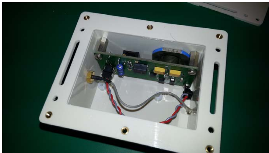
Figure 32: Specific power supply electronic board for WDC
