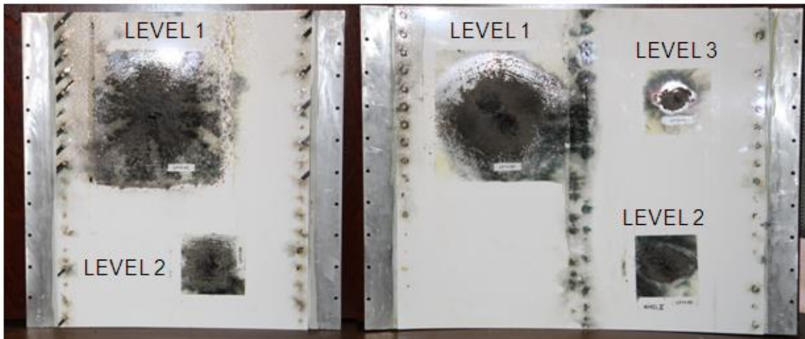
Figure 19. Multifunctional coupon (left) and reference coupon (right) tested
