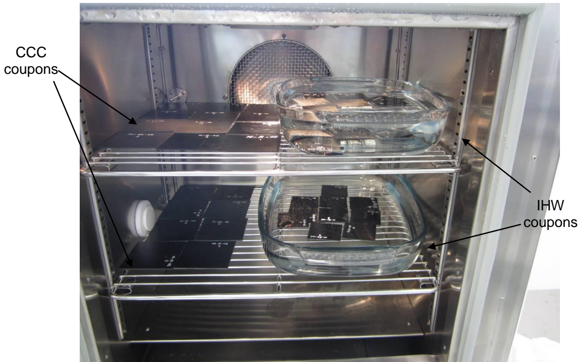
Figure 17. Interior of climatic chamber with CCC and IHW coupons
