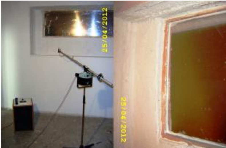
Figure 20. Left) Aluminum test specimen mounted in the wall of the double partition room; (right) detail of the installation of the test specimen
