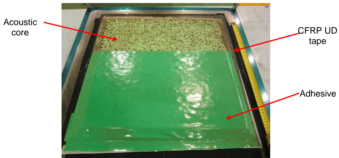
Figure 8. Manufacturing of sandwich panel with Hexweb® acousti-core®
