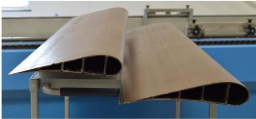
Figure 2: DEAMAK left- and right-hand wing Krueger panels for BLADE aircraft after demoulding at ASCO in May 2016
