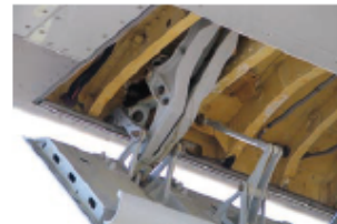
Example of one of the two Krueger flaps (below), designed and manufactured by ASCO Industries for flight testing on a modified A340-600 by Airbus (above).
