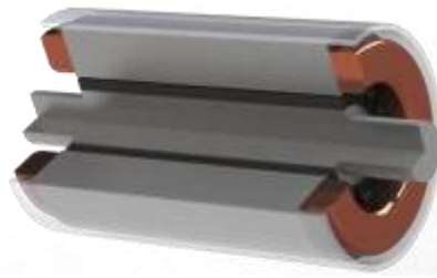
Circumferential Segmentation DL FSCW topology
