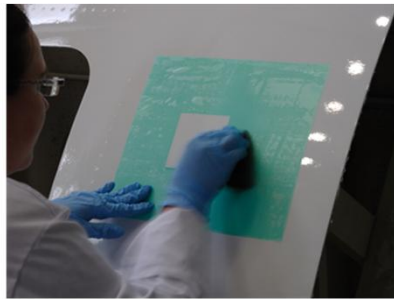
b. Application of stencil and paint
