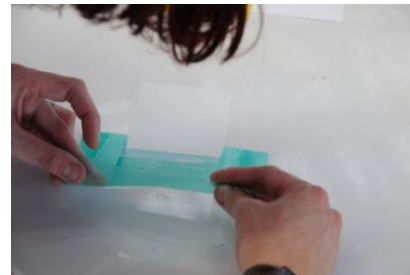
d. Removing of stencil; riblet test patch is ready
