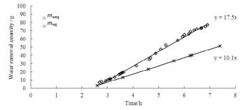
Comparison between  $m_{\text{weg}}$  (water removal by both EO and gravitational force) and  $m_{\text{wg}}$  (water removal only by gravitational force) when applied voltage E is 17 V cm<sup>-1</sup>.
