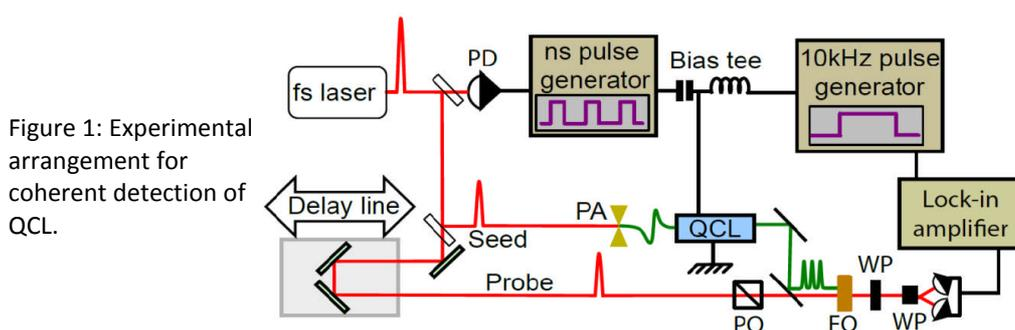
Figure 1: Experimental arrangement for coherent detection of QCL.
