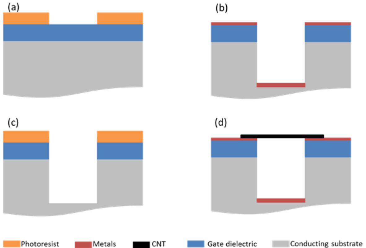
Figure 4: Summary of the process flow. (a) Patterning photoresist using deep-UV illumination, (b) two-step dry etching for trench creation, (c) metal evaporation for self-aligned contacts, (d) CNT growth.
