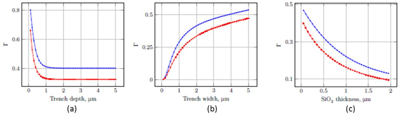
Figure 3: Simulation results on the effects of (a) trench depth, (b) trench width, and (c) gate dielectric thickness on the gate coupling ratio
