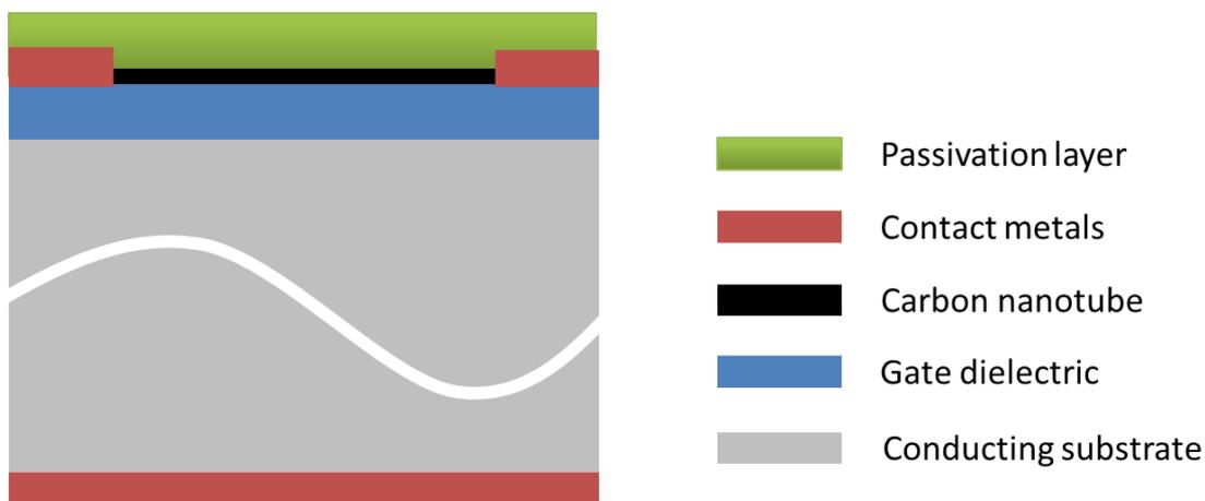
Figure 1: Schematic of a typical carbon nanotube field effect transistor
