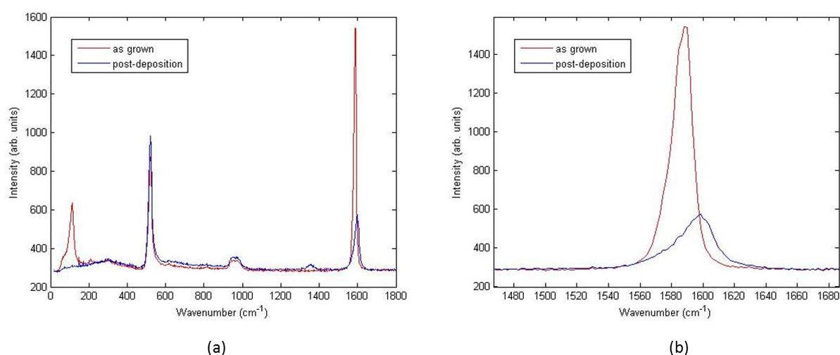
Figure 6: Raman spectrum of an example nanotube before and after insulator deposition. (a) shows the full spectrum, (b) zooms in on the G-peak shift and broadening.
