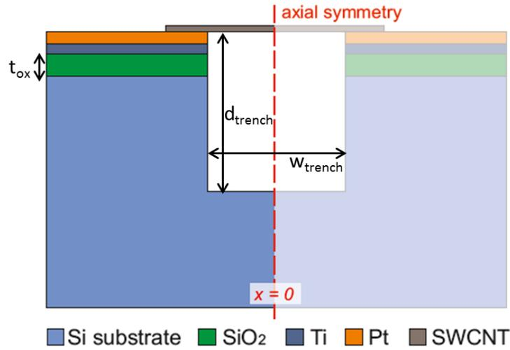
Figure 2: Trench structure as simulated. For reduced complexity, only half of the structure was simulated (to the left of the axis of symmetry).  $t_{ox}$  is the gate dielectric depth,  $d_{trench}$  is the depth of each trench and  $w_{trench}$  is the width of each trench.
