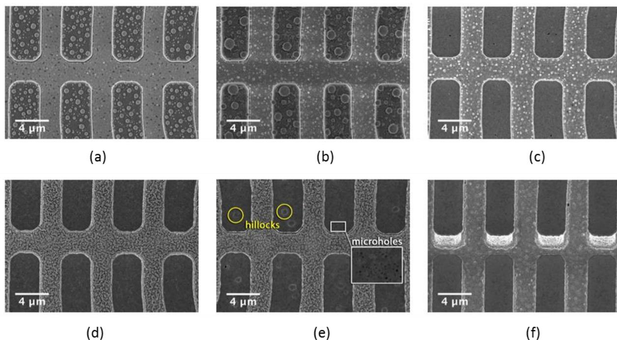
Figure 5: SEM images summarizing the metal stack optimization study. The thicknesses of the Ti/Pt stack are (a) 10/100nm, (b) 10/150nm, (c) 10/200nm, (d) 10/250nm, (e) 5/200nm, and (f) 10/200nm (tilted view).
