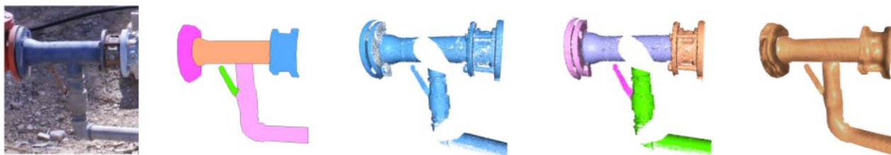
Figure 4: Given a partial 3D scan and a 2D photograph (left), we lift 2D shape structures into 3D yielding a faithful textured mesh reconstruction (right).
