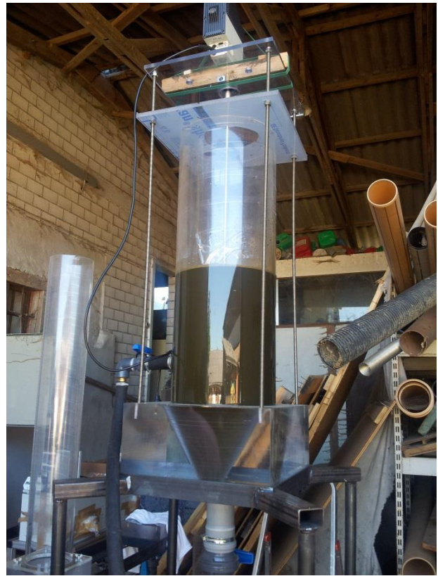
Heat exchanger and struvite precipitation system of EfficientHeat pilot plant
