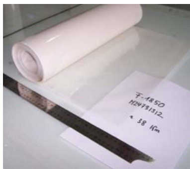
Figure III–2: Membrane roll of fumapem® F-1850 (length 38 m, width 50 cm, Lot No M24731312) on white PET foil as backing.
