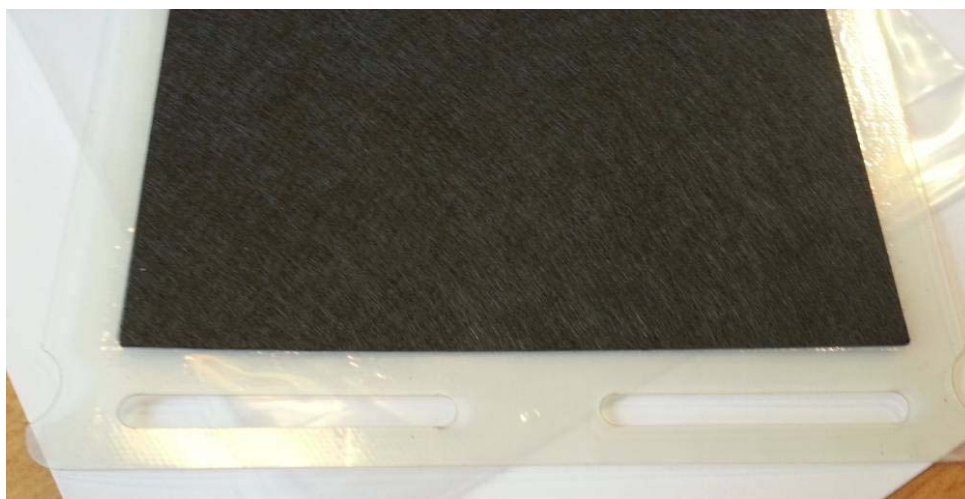
Figure V–2: Picture of the scaled up IRD 180 cm 2 7-layer DMFC, based on F1850.
