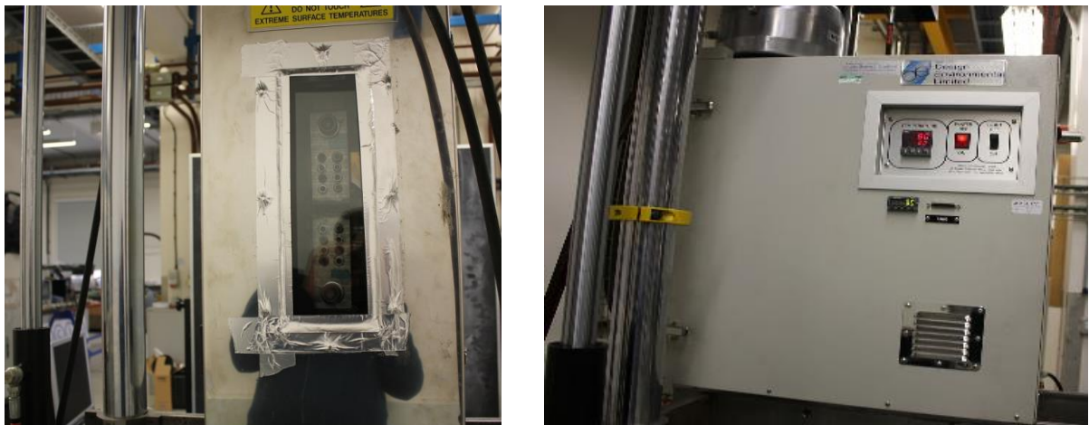
Figure 23. Mechanical testing setup for high temperature (Front and side view of the chamber)
