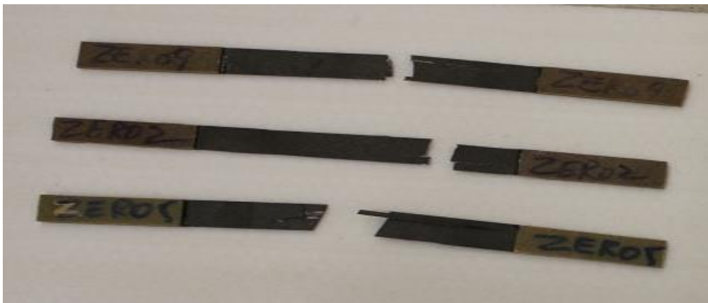
Figure26. Failure surfaces of 0° orientation specimens for dry test at 80 °C
