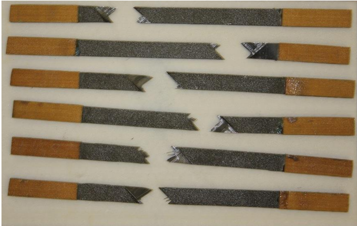
Figure17. Failure surfaces of \pm 45^\circ orientation specimens for wet test at room temperature
