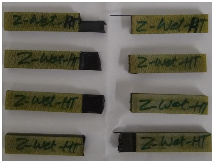
Figure 58. Failure surfaces of 0° orientation specimens for wet tests at 80 °C
