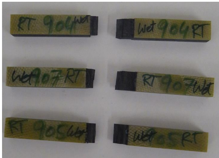
Figure 53. Failure surfaces of 90° orientation specimens for wet test at room temperature
