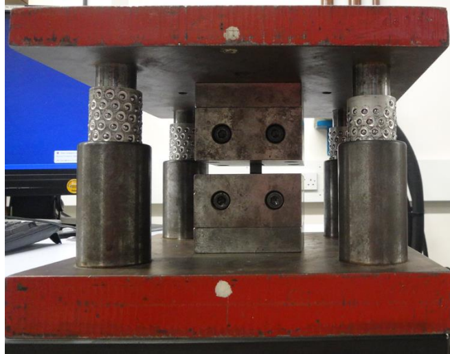
Figure 41 Compression jig used for mechanical testing (Top and side view)
