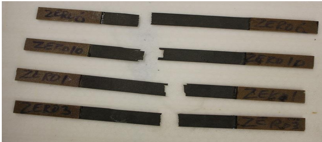
Figure27. Failure surfaces of 0° orientation specimens for wet tests at 80 °C
