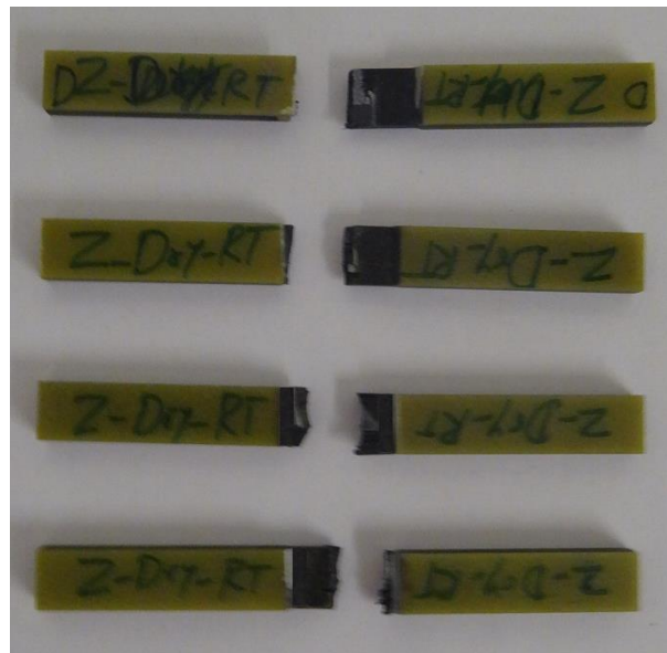
Figure 44. Failure surfaces of 0° orientation specimens for dry test at room temperature
