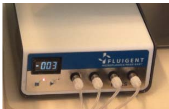
Figure 7.5. (left) OEM design and (right) Instrument of the Fluigent pressure control unit.
