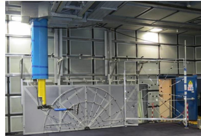
Figure 9 – Lateral, forward and linear far field microphone arrays with the near field traversing arm
