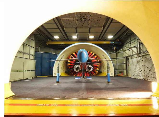
Figure 8 – Aircraft model in wind tunnel with microphone arrays
