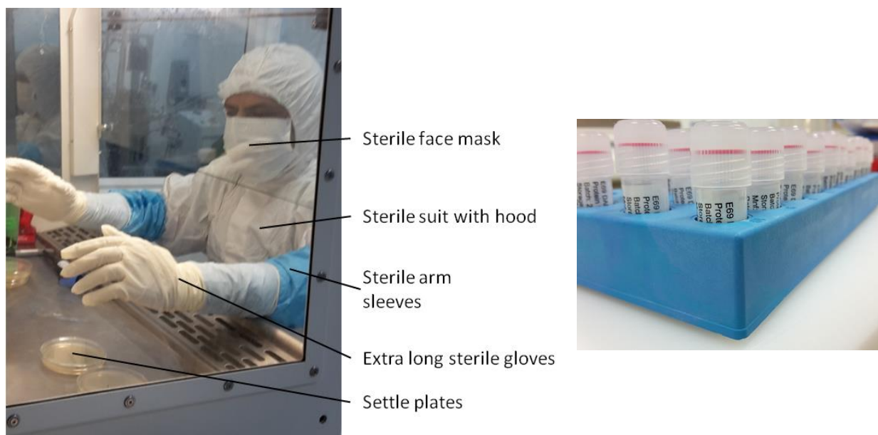
Figure 22: Preparation for final fill of E69 protein in the grade 'A' VLFH space (left) and Final fill vial rack for a GMP compliant batch.
