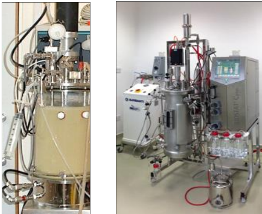
Figure 19: (Left) 10L Bioreactor for Process Development. (Right) 20L CIP Bioreactor in GMP Facility.
