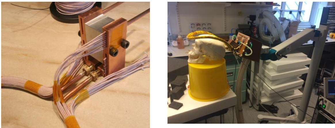
Figure 13: (left) Example of litz wire termination for head coil. (right) demonstration of mounted dished elliptical coil.
