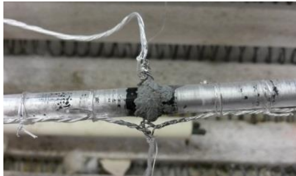
Ny/MT sealant silver degradation, but still acceptable performance
