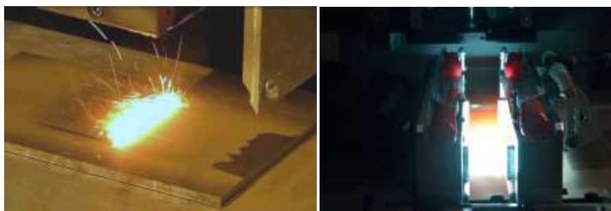
Figure 4. Laser sintering (left) and laser drilling (right)
