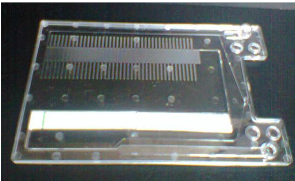
Figure 3.5. Layout of the PCR + OC chips for injection molding production and corresponding injection-molded polymeric chip.
