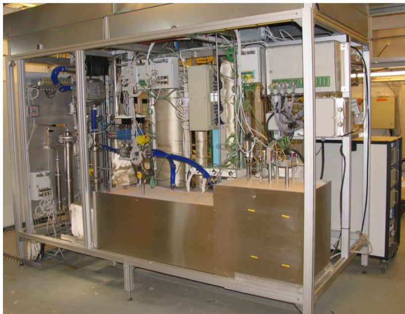
Figure 31. SOFC stack module installed and insulated in the in-house proof-of-concept in Helsinki.
