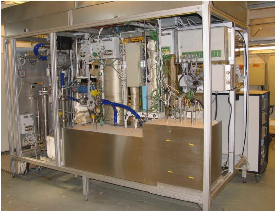
Figure 3. SOFC stack module installed and insulated in the in-house proof-of-concept in Helsinki.
