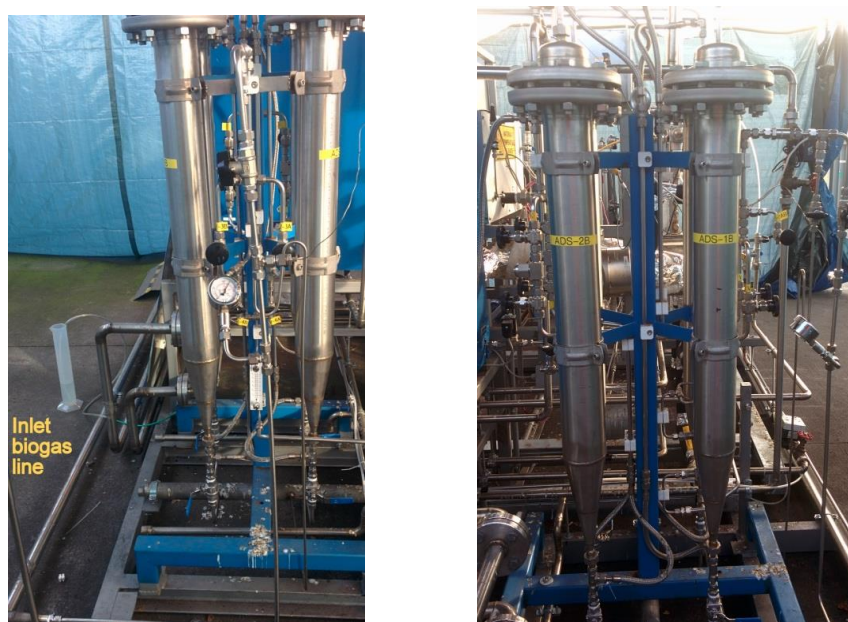
Figure 22. Biogas cleaning unit – frontal view and lateral view.
