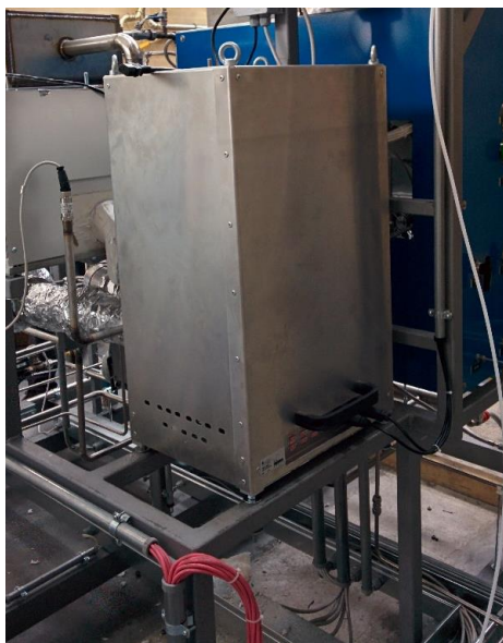
Figure 24. SOFC Stack installation.
