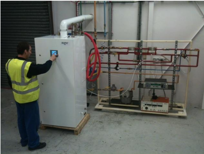
SIFC Power units being tested
