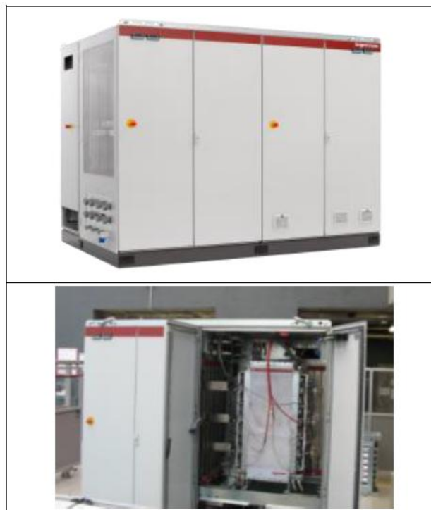
Figure 2 Power stack developed and test bench at Ingeteam labs
