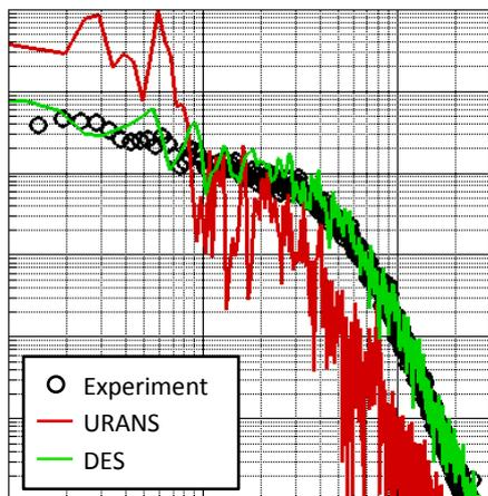
Figure 3: Comparison of surface pressure spectra between DES, URANS and experiment (with landing skids).
