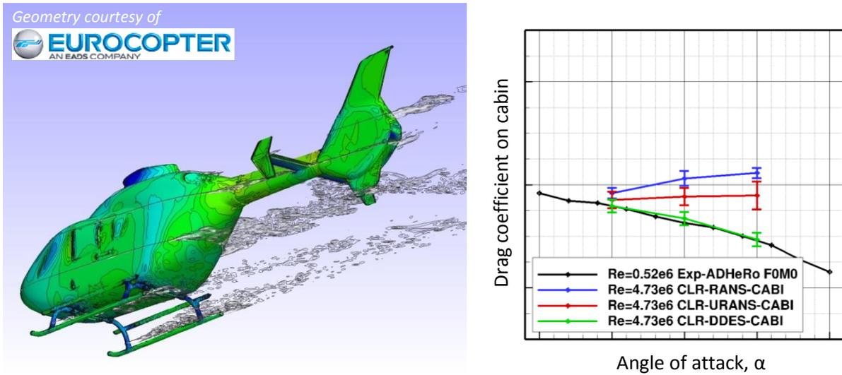
Figure 1: Snapshot of DES flow field (left). Comparison of drag coefficient on cabin between RANS, URANS, DES and experiment for configuration without landing skids (right).
