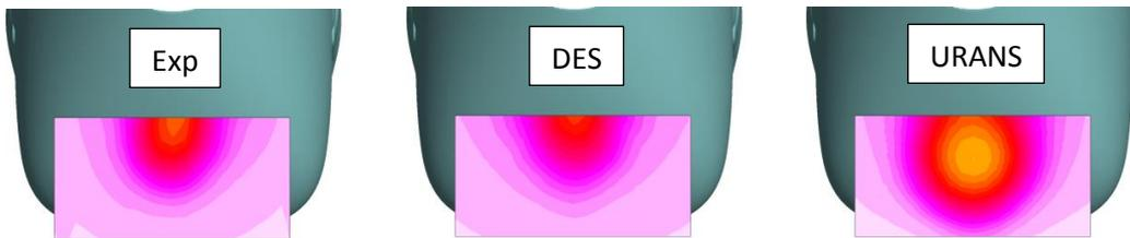
Figure 2: Comparison of mean streamwise velocity in the fuselage wake between experiment, DES and URANS for configuration without landing skids.
