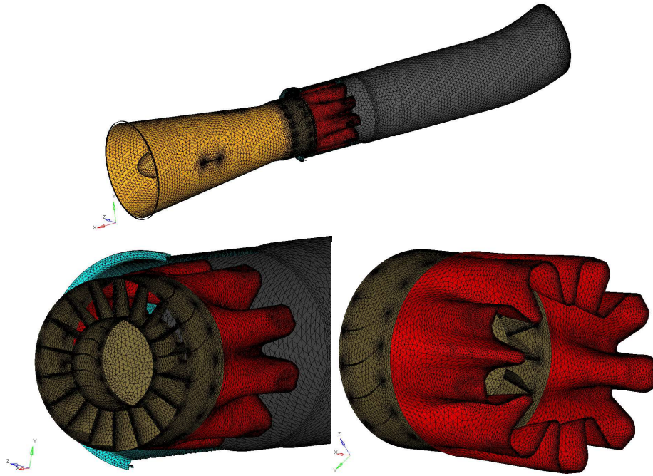
Figure 7: Details of the computational mesh used for validation of the AW101 exhaust numerical model.
