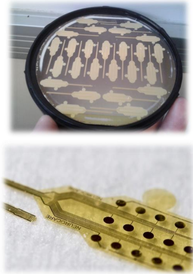
Figure 5: Left: 4-inch wafer with several implants during the fabrication process. Right: Finished devices showing the head of the implant with 16 transistors and the tail with the bond pads
