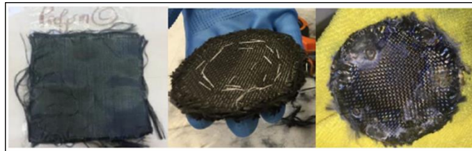
Fig. 8: SiC Nicalon fabric (left), hand-made preform (center) and infiltrated preform (right)
