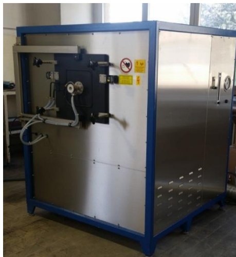
Fig. 9. Assembled MW-furnace for LSI of SiC foams.
