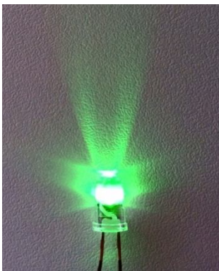
Packaged green emitting (11-22) semipolar LED
