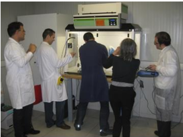
Figure 7. Measurements of airborne NPS during weighing (a) and Ink jet printing operations (b)
