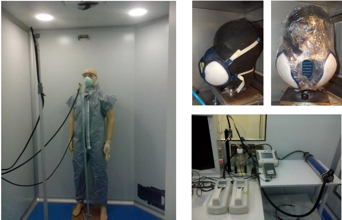
Figure 9. Manikin (a), Sheffield heads (b) and aerosol generator (c) used for effectiveness testing
