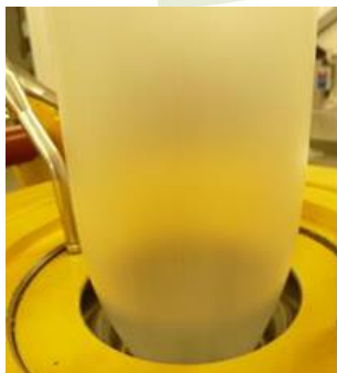
Figure 9. Blown film with cellulose nanofibre composition.
