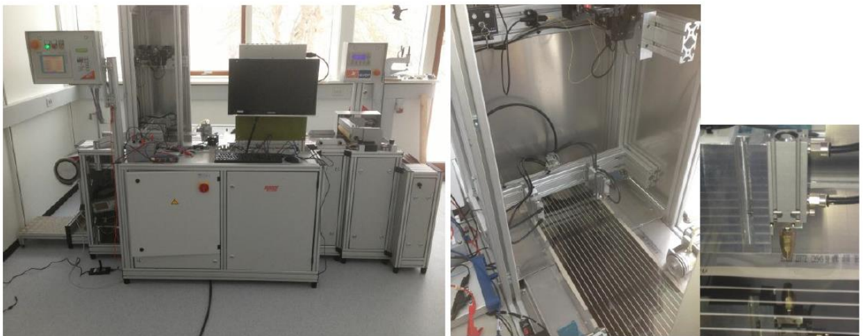
Figure 2. Photograph of the LBIC setup integrated in a R2R line.
