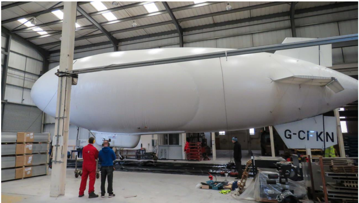
Figure 3: 23m long helium filled airship by Lindstrand Technologies Ltd, with an electric motor and remote-control.
