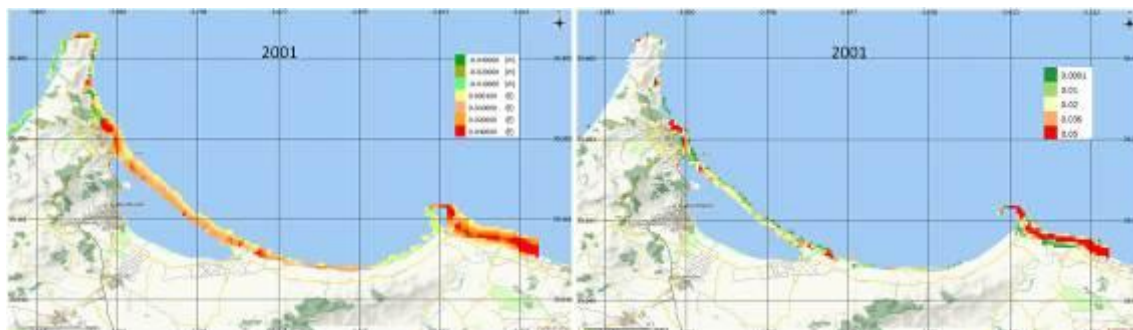
Fig. 16. Erosion potential for longshore sedimentary transport at Nador, based on the median value of wave stress on bottom, left and 90 th percentile, right ; (W) - greenish colours correspond to sedimentary transport towards the West, while (E) and others colours corresponds to transport towards the East.
