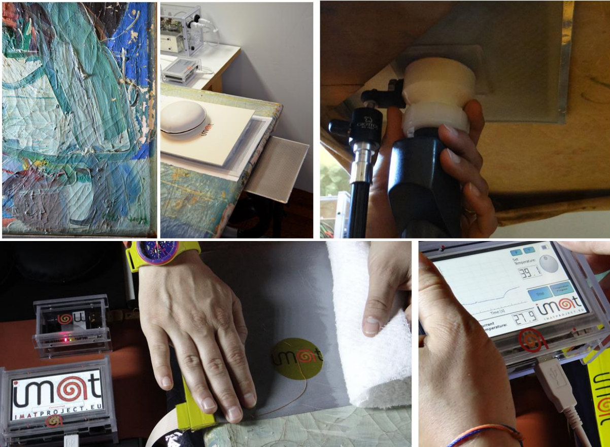
Figure 67 – Photo detail of the surface in oblique light; demonstrative photo of the suction platen, IMAT-B, thermal isolation layer, foamcore; photo of the suction scupper positioned under the canvas; IMAT positioning on the painting and IMAT touchscreen with temperature settings.
