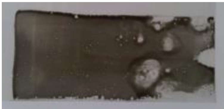
Figure 24 – final heater based on translucent silver coated heating fabric
