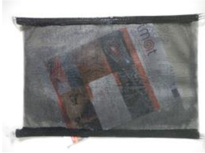
Figure 21 – an example of early transparent heater with fine mesh
