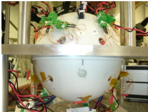
Figure 3: Laboratory prototype of a Reaction Sphere realized with a plastic stator (diameter 20 cm).
