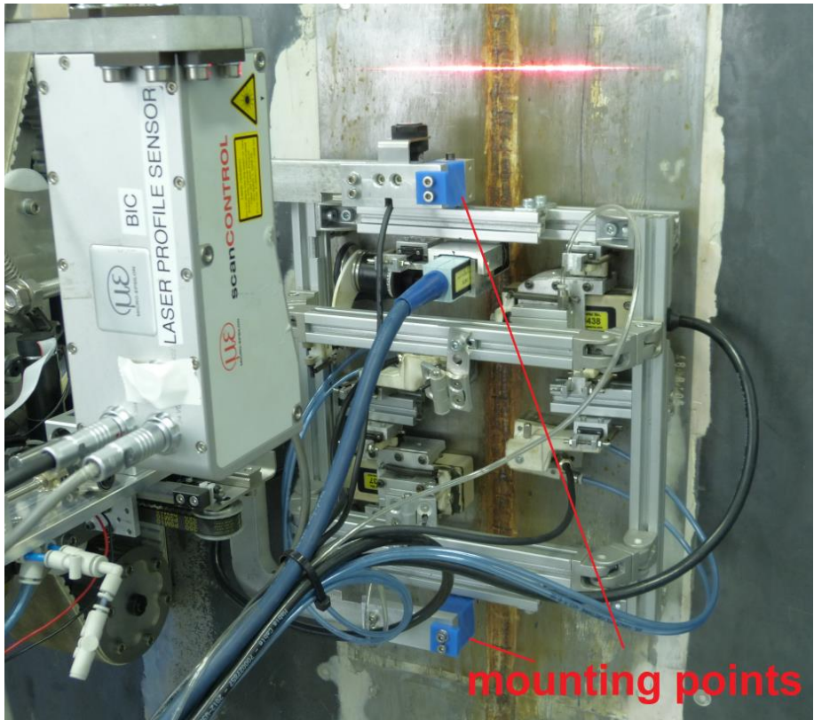
Figure 17: Mounting points of the sensor holder on the robot
