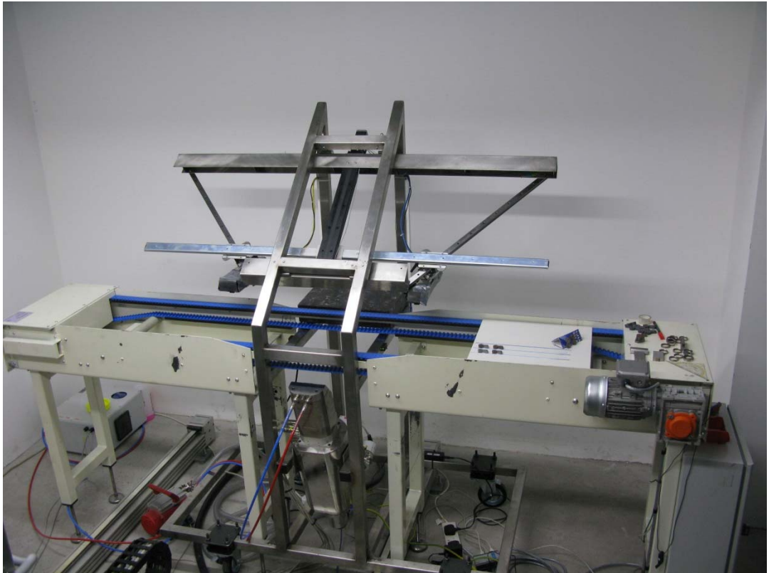
Figure 4 AutoInspect system in TWI's radiography bay
