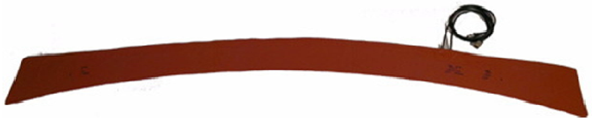
Figure 5 A 3 meter long and variable width blanket consisting of 2 heating zones, 4 thermocouples and 2 cables for connection of power and thermocouple sensors. The main heating blankets specification is: Operating ambient temperature >0^{\circ}\text{C} , Power density of 2500 watts per square meter and a maximum blanket area of 4 Square meters.
