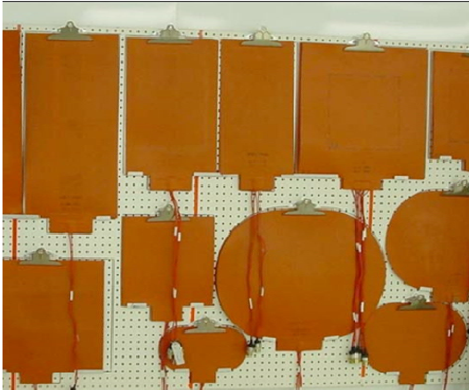
Figure 4 Heating blankets for use with different size and shape damage areas
