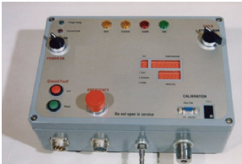
Figure 7 Robust, “push-button” conductive heating console for use in-situ repair of wind turbine blades
