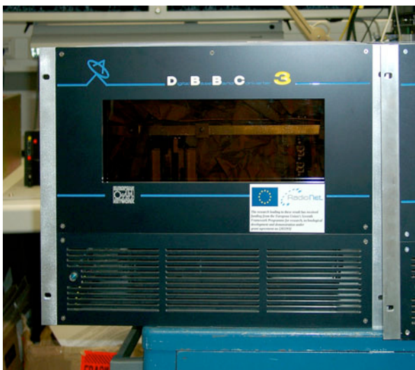
Front view of the DBBC3 – a VLBI backend developed in JRA DIVA.
