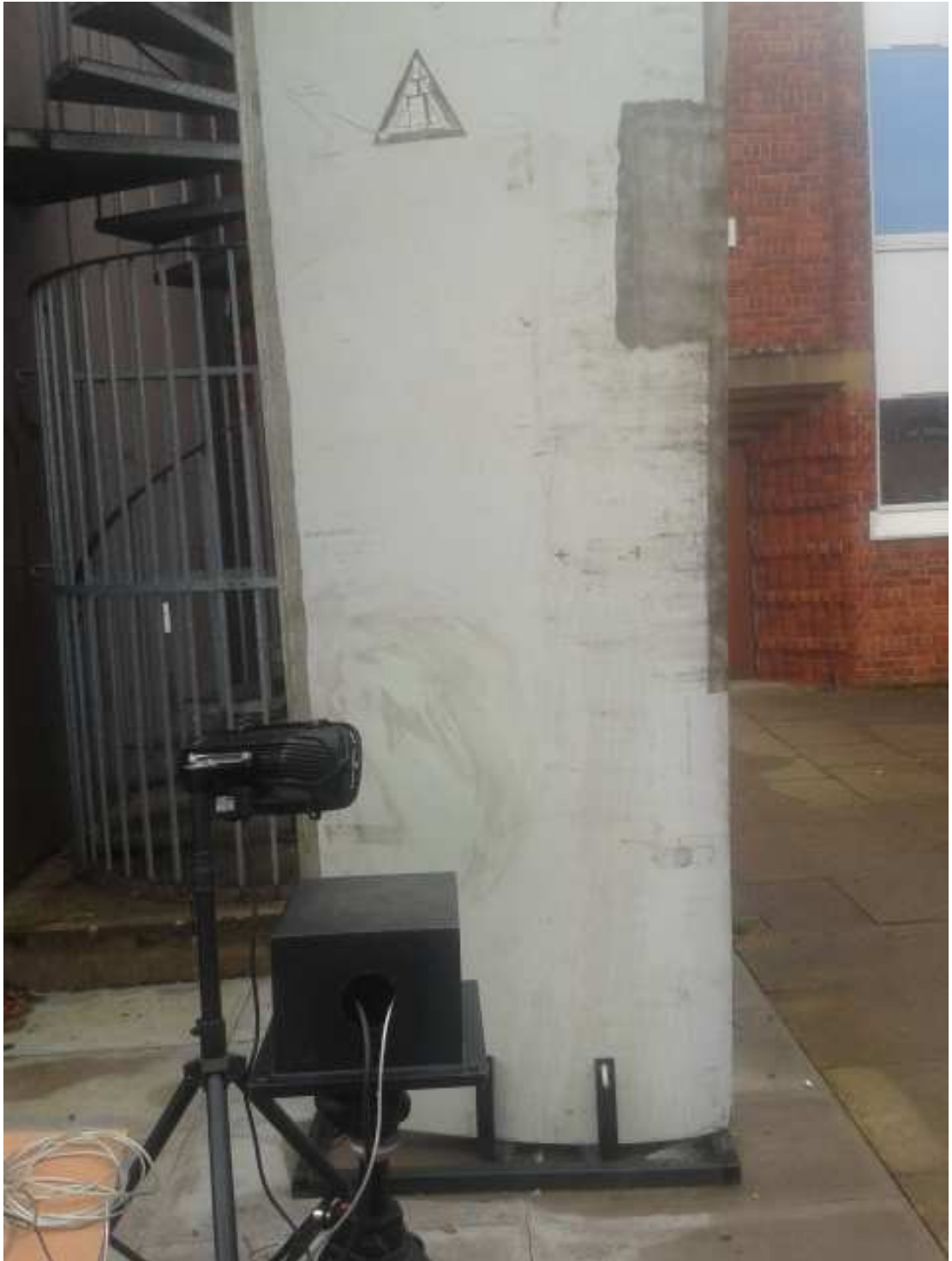
Figure 77 A standing 4m long WTB, an infrared heating lamp and the shearography system in an outdoor test.
