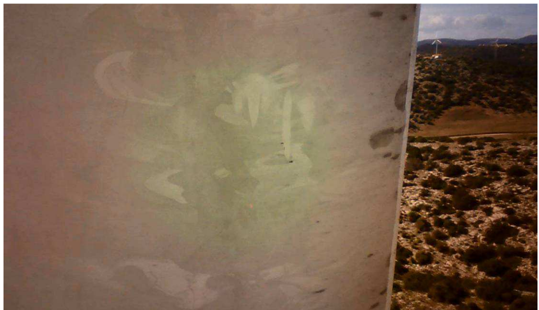
Figure 91 Laser illuminated area on the WTB which was captured by the surveillance camera on top of the shearography box.
