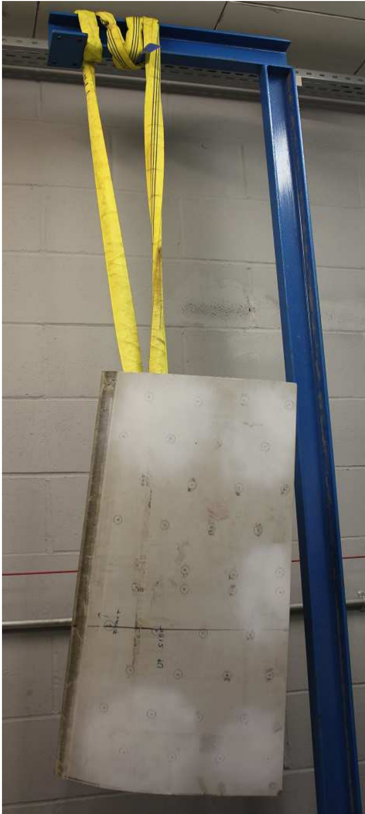
Figure 42 Experimental setup for rigid body motion measurement of a WTB suspended from a test frame.
