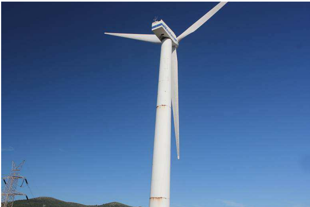
Figure 93 A full image of the Vesta V47 wind turbine in which the WTBs have a length of 23m.
