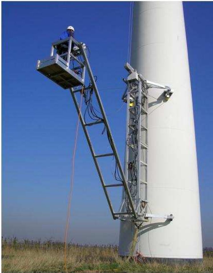
Figure 3 A magnetic climbing robot platform (Courtesy of BSR)
