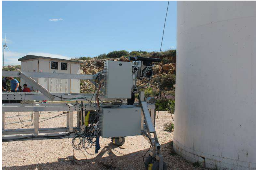
Figure 85 Attachment of the lifting cable on the main winch mounted on the platform.
