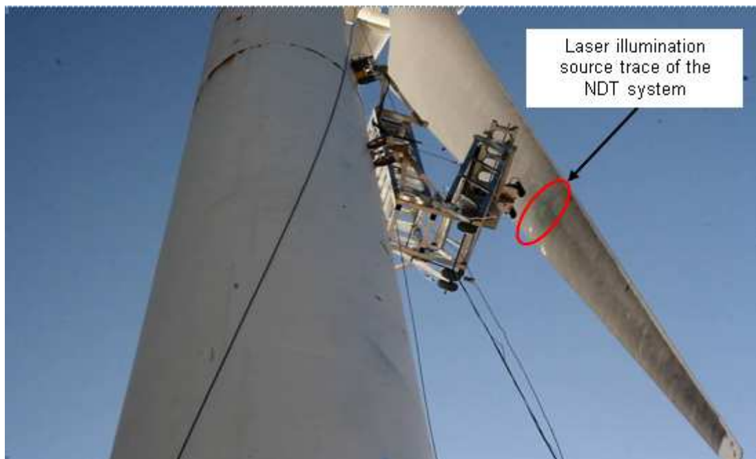
Figure 89 Robot arm opened to enable the shearography system to achieve the correct distance from the WTB. [Note that the green spot ahead of the heating lamps is the laser illuminated area where the inspection will be carried out.]
