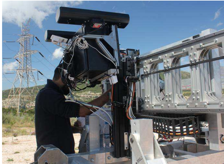
Figure 83 Mechanically assembling the shearography system onto the robotic platform.
