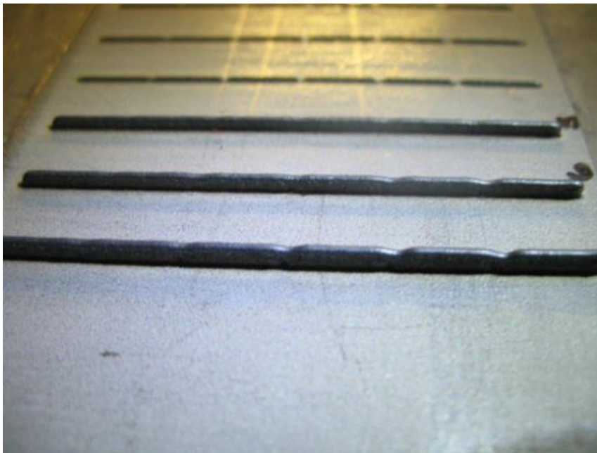
Figure 15 Single line deposits to develop defects (In 718)
