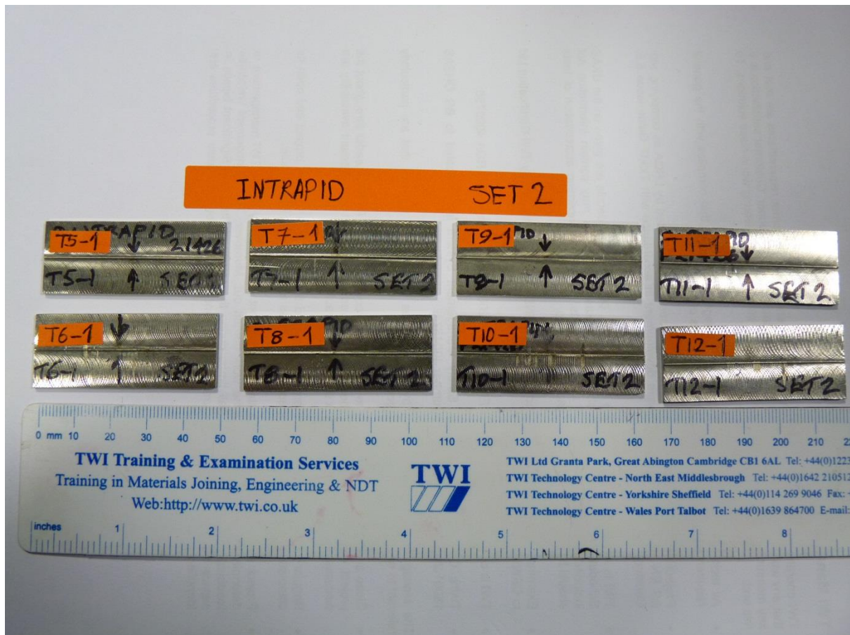
Figure 6 Type 2 Samples Manufactured by Electron Beam
