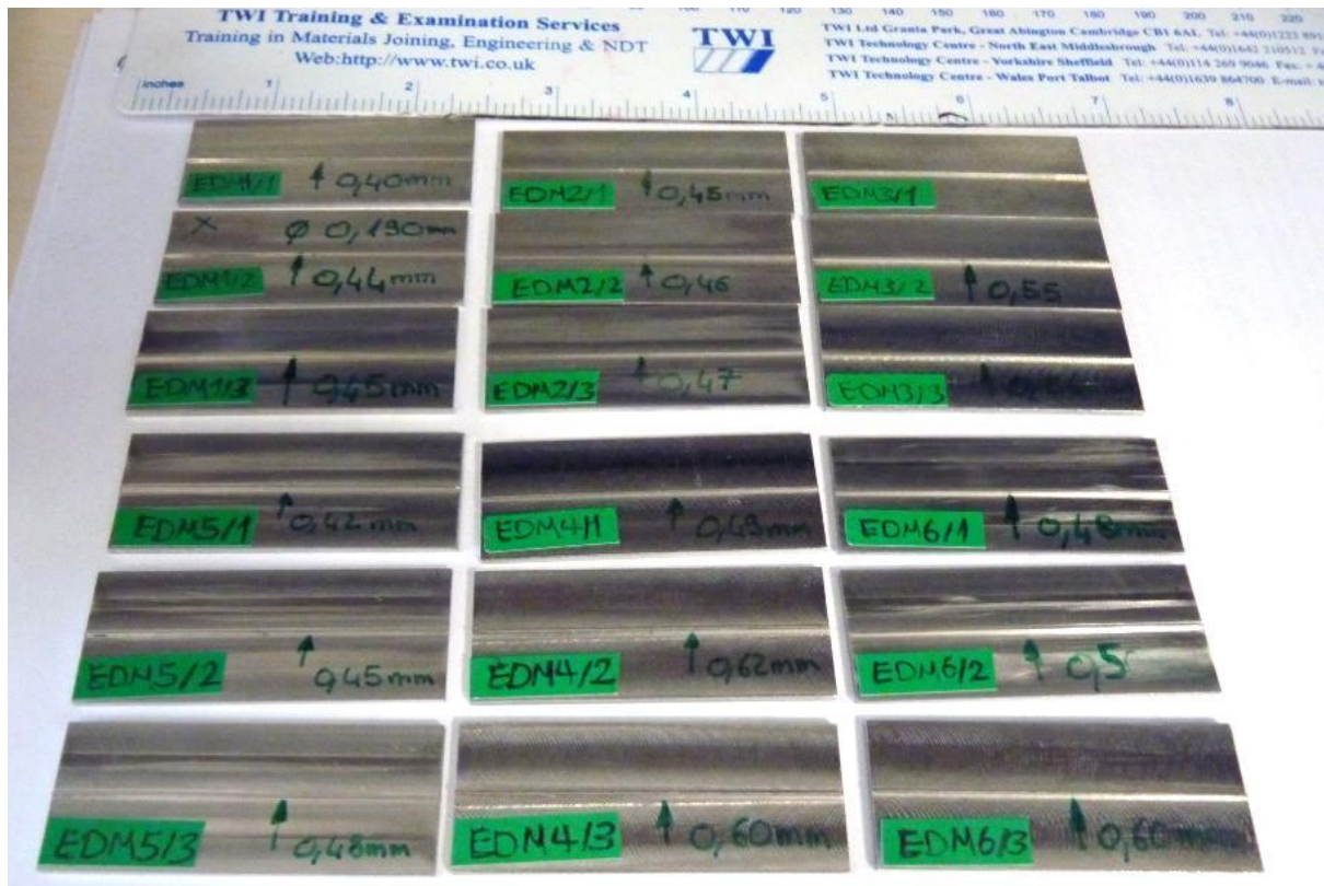
Figure 8 Samples made by EDM Microdrilling
