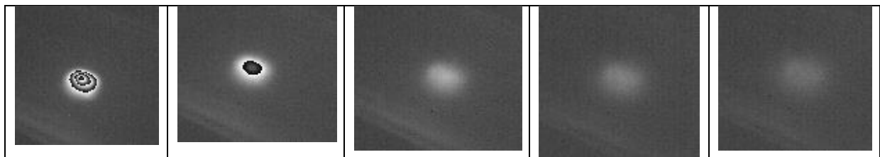
Figure 75 Recording of laser pulse striking surface at 20mSec intervals during and after laser pulse
