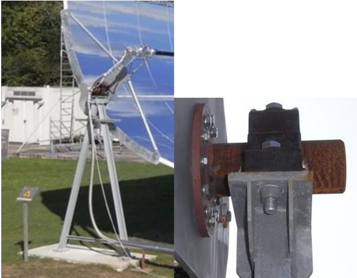
Figure 14: West end of collector row and bearing with shaft for attaching the prototype
