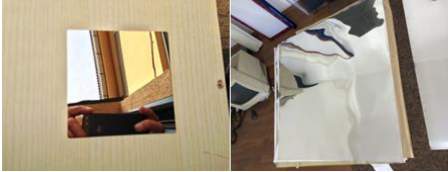
Figure 13: Deposition of PVD Ag reflective coating on thin glass substrate as protective layer (left photo) and on polymer foils as protective layer (right photo)
