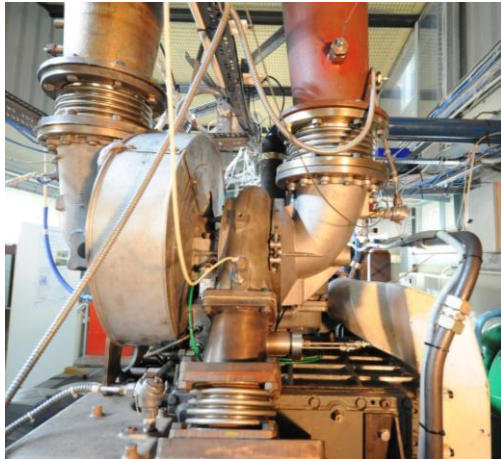
Figure 25: Turbocharger of NTUA-LME research engine (left) & trajectory of measured data during surge cycles (right)
