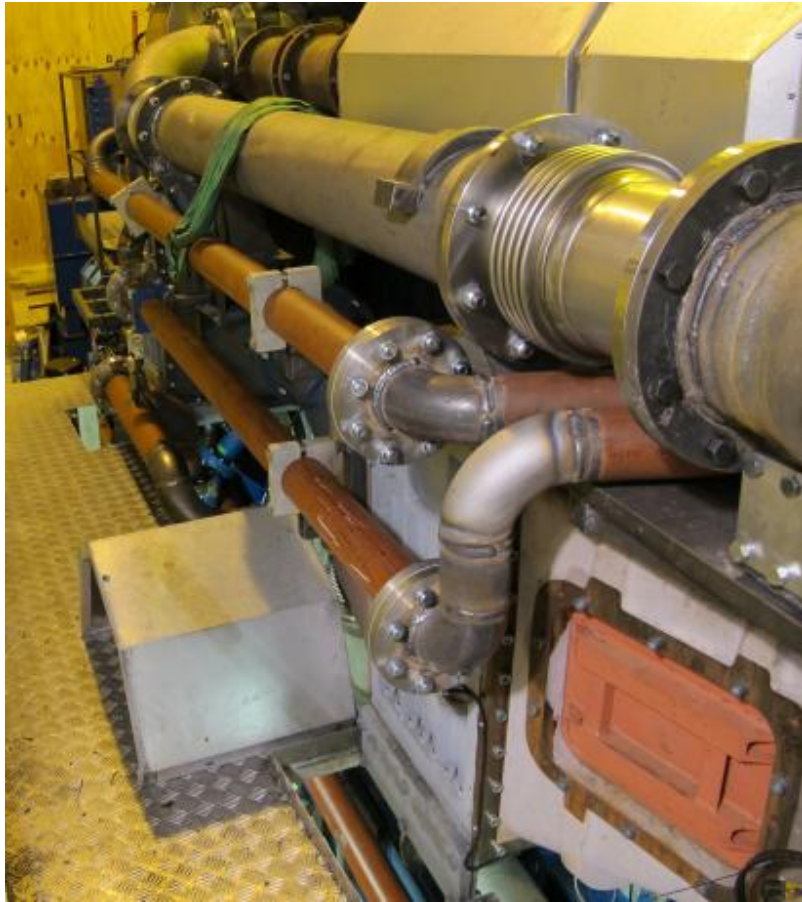
Figure 10: 4-stroke engine direct gas injection investigation test platform
