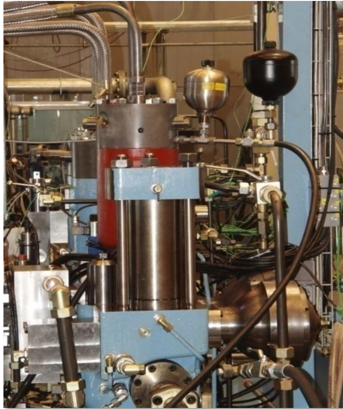
Figure 62: Test of JiT-WiF basic concept at injection test rig
