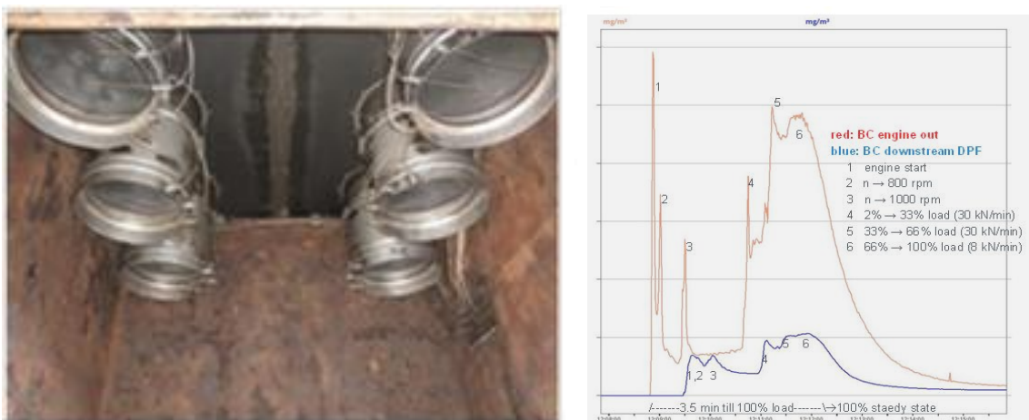
Figure 61: DPF installation(left) and transient (right) black carbon emission up- (red) & down-stream (blue) of DPF
