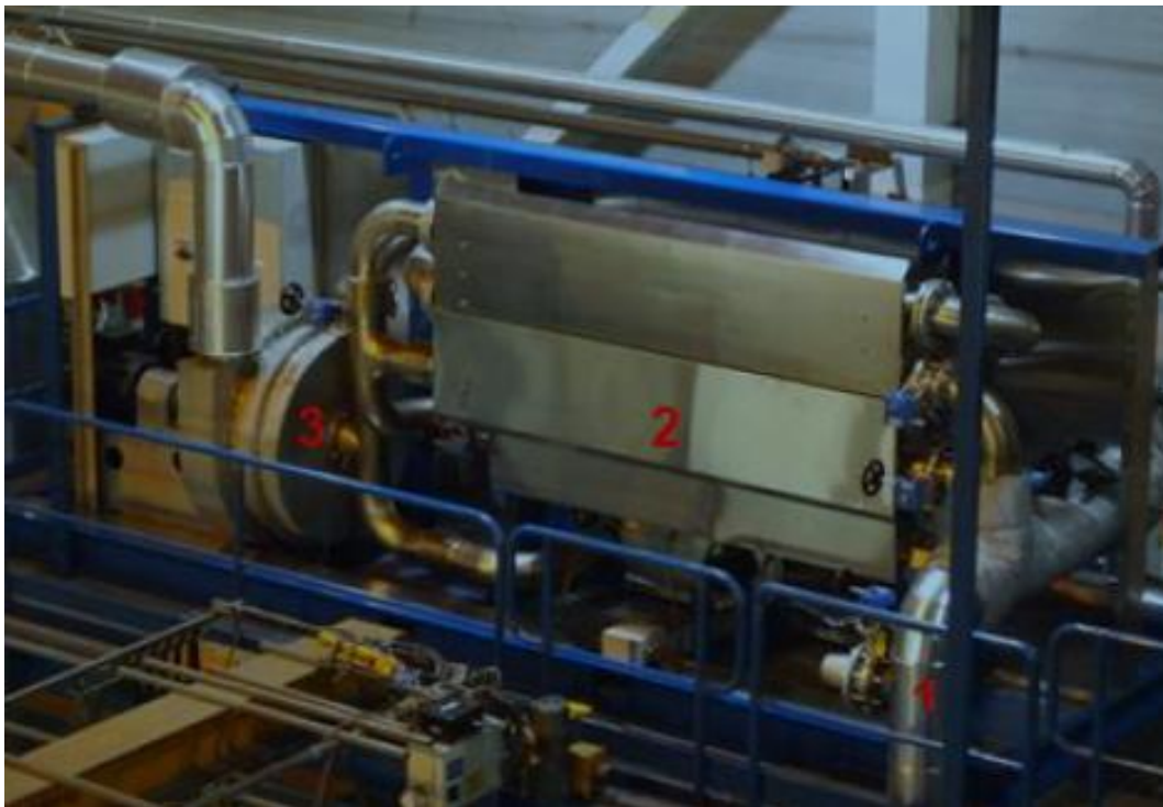
Figure 23: Side view of developed SCR bench, showing inlet (1), heating and cooling (2) and flow producing fan (3).
