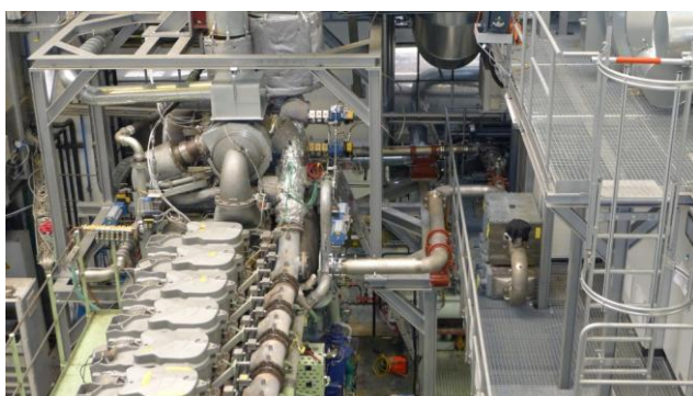
Figure 24: 2-stage turbocharging and ETB12 set-up at 4-stroke test engine 6L32/44-CR (left) & NO x reduction vs. blower speed at constant flap position (right)
