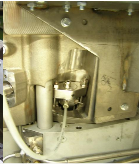
Figure 52: Optical probes in a multi-fuel single-cylinder engine
