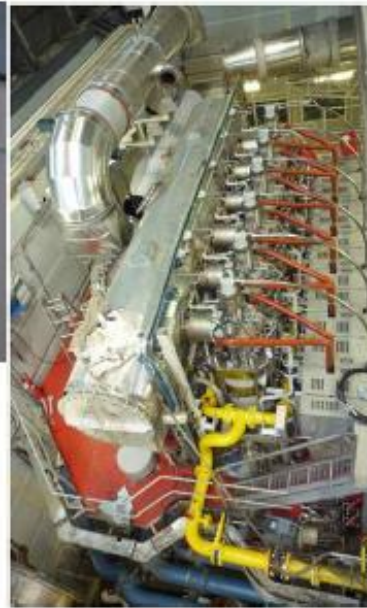
Figure 51: 2-stroke engine “low temperature combustion” with DWI
