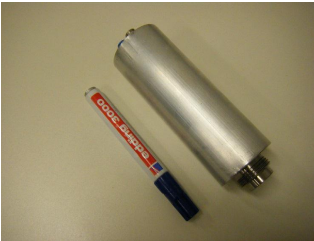
A 40 normal liter Cool gas Generator for terrestrial applications [APP]
