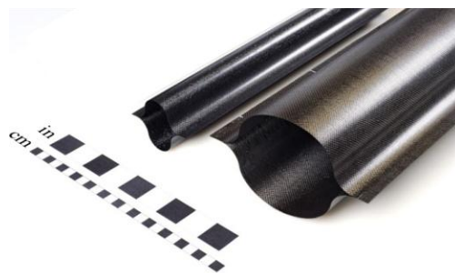
Figure 4: Comparison of a Gossamer-2 boom (right) and a Gossamer-1 boom (left) built at DLR
