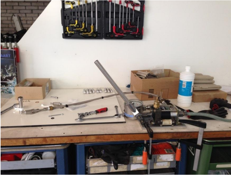
The DM SMCGG (left) undergoing pressure tests with the pump to the right
