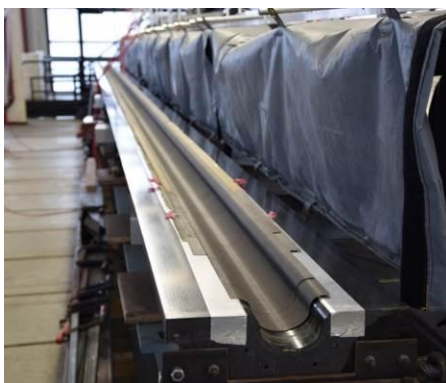
a) Cured 14 m boom half shells in the mould-tool
