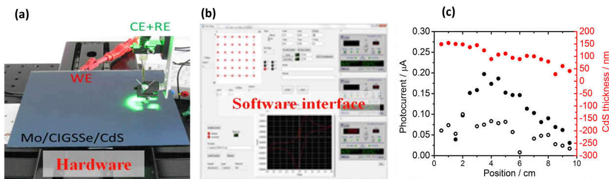
Figure 16: (a) View of the PEC mapping tool hosting a CIGSe/CdS sample being analysed. (b) Software interface. (c) Results of a PEC mapping test on a CIGSe sample with graded CdS thickness to assess measurement reproducibility: full and hollow black dots correspond to first and second set of measurements, respectively.
