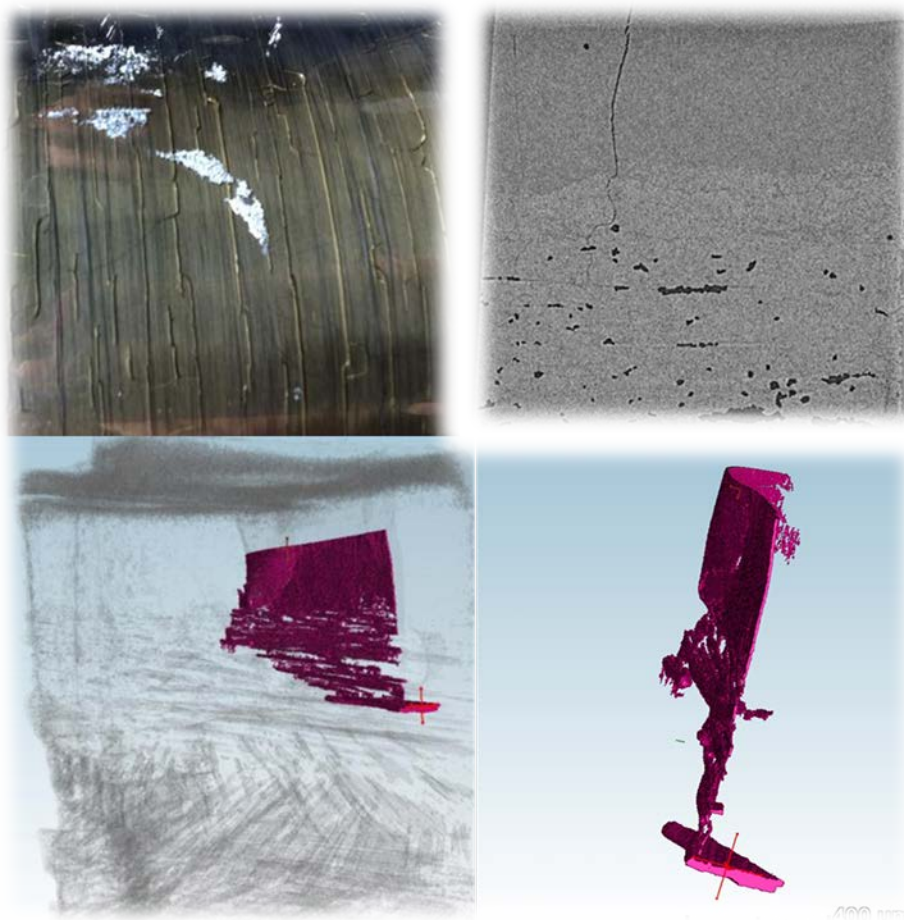
[Fig.8] An example of multi-scale structure characterisation: from full component (top left), to micro imaging (CT shot, top right), to isolation and quantification of crack parameters (bottom pictures)
