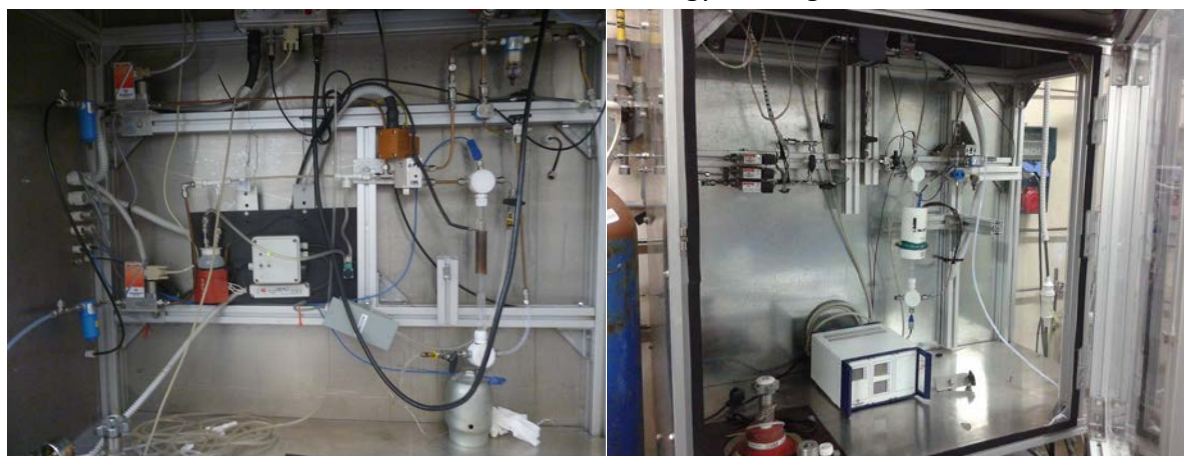
[Fig.21] Test bench (Gas clean-up rig for constant humidity shown in left image and gas clean-up rig for variable humidity shown in the right image)
