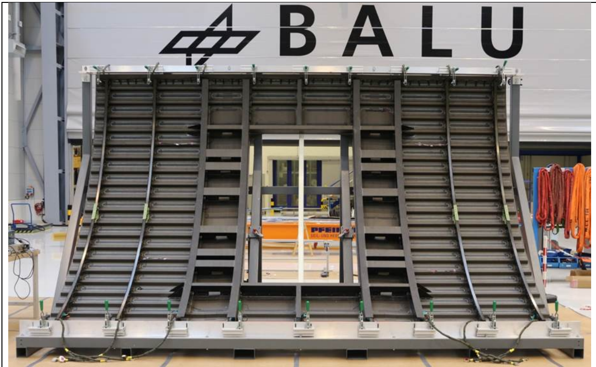
Figure 2: SARISTU 5 X 4m self-sensing Door Surround Structure at DLR
