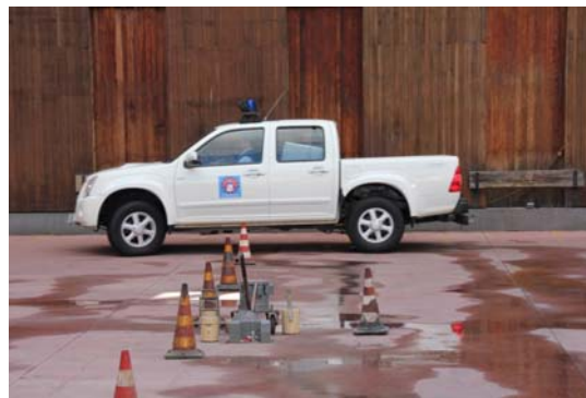
Figure 25: Civil Protection car equipped with the sensor tag passing near the radioactive sources in Naples fire brigades headquarters.
