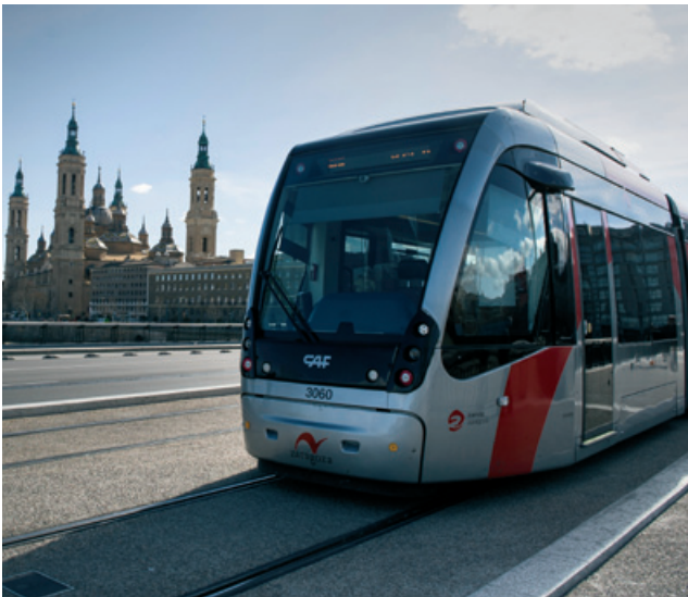
Tram in Saragossa powered with onboard energy storage
