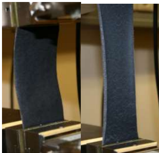
Figure 6: Picture of the leather coated side of one sample during stress strain measurement. The new material can be stretched up to 40 - 50%.
