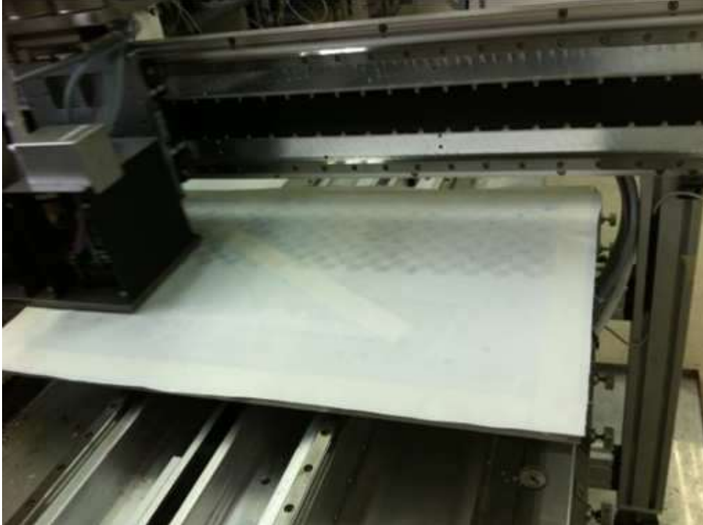
Figure 19: Digital Functionalization. Experiment printing a checked pattern with finishing agent
